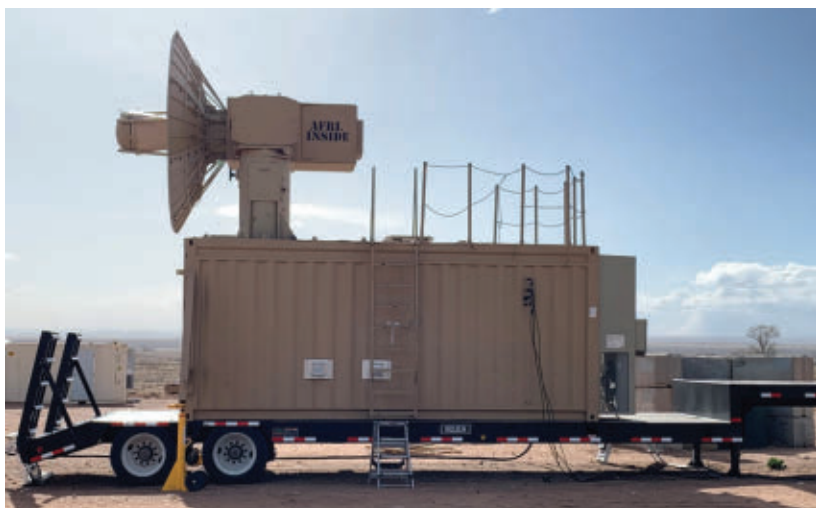
▲ The Tactical High-power Operational Responder, or THOR, a high-powered microwave counter drone weapon, stands ready to demonstrate its effectiveness against a swarm of several targets.
